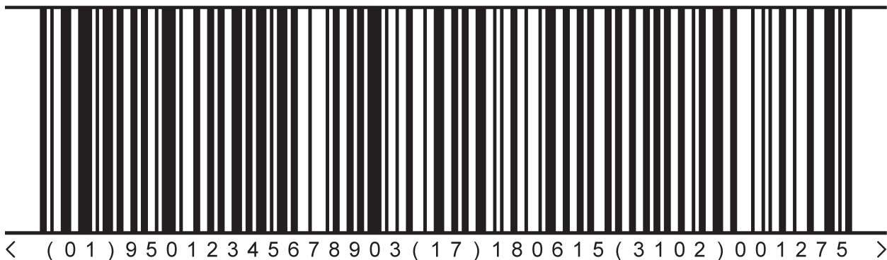
The data in this barcode provides the information that the GTIN is 95012345678903, that the product's net weight is 12.75 kilograms, and that the expiry date is 15th June 2018.
