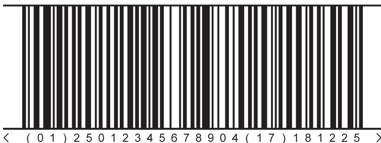
GS1-128 barcode with X-dimension of 0.50 mm
